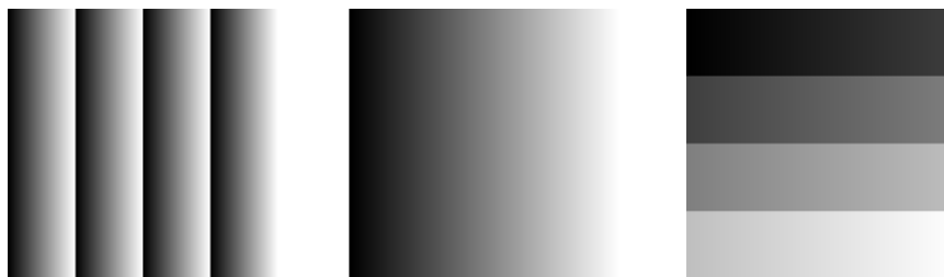
Figure 4.21: Ramp test images: 8 bit output (left), 10 bit output (middle), 12 bit output (right)
