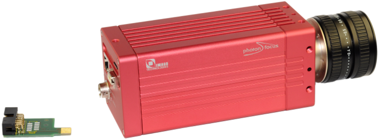
Figure 2.2: SM2-JTAG adapter and camera
