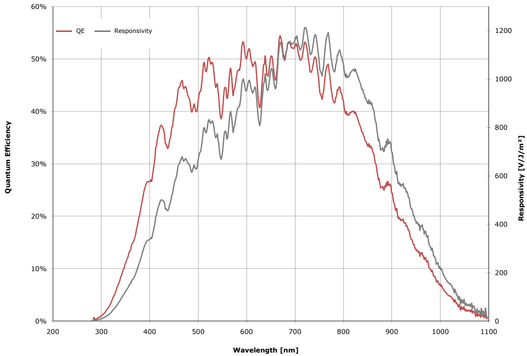
Figure 3.3: Spectral response of the A1312 CMOS monochrome image sensor (standard) in the SM2-D1312-T16455 camera series
