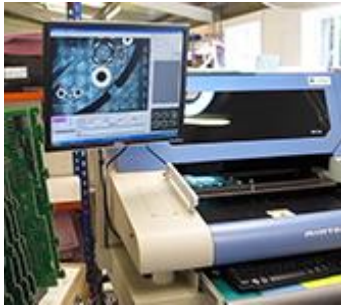
AOI: PCB Inspection
